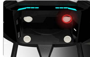
Optical collision warning from Ultrasonic sensors
